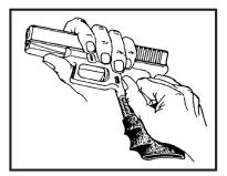
4. The grip must be pulled onto the firearm frame. Slip your fingers under the sleeve and grab the edge. Pull upwards onto the firearm. Do not pull outwards any more than necessary. Do this a little at a time alternating from right to left, back and forth, inside and out, whatever it takes until the grip is to its desired height.
