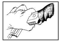
2. Begin by holding the firearm as shown. At the rearmost corner, cover the frame with the HANDALL Jr. Make sure it is right side up. Look for the (up<sup>↑</sup>) inside the grip.
