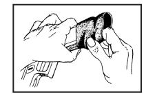
3. Next, pull the sleeve towards the front of the firearm until the finger groove ridge is over the front corner of the frame. The HANDALL Jr. is designed to fit tightly and much force may be required to complete this step. The sleeve should be stretched as evenly as possible. The rubber is very durable and tear resistant although care must be exercised not to gouge, cut, or pull excessively on the edges of the sleeve, as a tear may develop.
