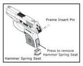
**2.** Remove the "Hammer Spring Seat" by depressing the tab through the hole at the rear of the frame while pulling the "Hammer Spring Seat" from the pistol.
