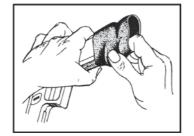
3. Next, pull the sleeve towards the front of the gun until the finger groove ridge is over the front corner of the frame. The HandAll is designed to fit tight and much force may be required to complete this step. The sleeve should be stretched as evenly as possible. The rubber is durable and tear resistant although care must be ecercised not to gouge, cut, or pull excessively on the edges of the sleeve as a tear may develop. Be cautious of sharp edges.
