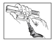
4. The grip must be pulled onto the gun frame. Slip your fingers under the sleeve and grab the edges. Pull upwards onto the gun. Do not pull outwards any more than necessary. Repeat this a little at a time alternating from right to left, front to back, until the retention tab is touching the lower corner of the receiver. Insert retention tab into corresponding recess and continue pulling sleeve onto receiver until HandAll is clear of the magazine well and retention tab is fully seated.
