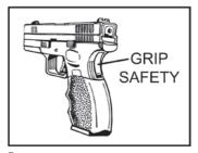
**5.** Verify that the installed sleeve does not interfere with the grip safety.
