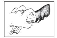
Start by holding the gun as shown. At the rearmost corner, cover the frame with the top edge of the HandAll sleeve. Note: Warming the HandAll will make it stretch with less effort and make the installation somewhat easier.
