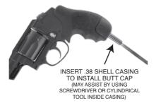
**9.** It is not necessary to remove your Hogue rubber grip for routine cleaning. If you need to remove it for further maintenance, simply insert .38 special shell casing (or prying tool) back into round cavity of butt cap to release it.
