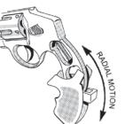
6. It is not necessary to remove Hogue rubber Bantam grip for routine cleaning. If you need to take it off for further maintenance, spread the bottom of the grip with the Hogue Bantam tool. Insert it just to the side or below the stock pin. This action will release the grip from the stock pin. Then simply slide if off while the tool is in place. Be careful not to spread the grip any further than is necessary to disengage the stock pin.
