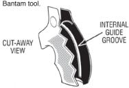
**5.** Continue sliding the grip onto the frame fully until the stock pin "snaps" into the corresponding internal stock pin holes. If necessary, squeeze grip together until
