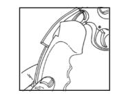
5 MONOGRIP<sup>®</sup> should be guided up behind the trigger guard, then pivoted to cover the frame straps. The grip must mate with the semi-circular loops at the top of the gun handle. MONOGRIP<sup>®</sup> must be fully seated on the frame before inserting mounting screw.
