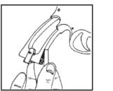
Your MONOGRIP® is designed to fit an average size firearm frame. However, frame dimensions do vary slightly from firearm to firearm. It necessary, your MONOGRIP® can be adjusted by placing small shim(s) of tape (as shown) on the lower corner of the front strap. Add or subtract tape until grip is flush with backstrap.
