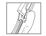
4 Mate the firearm handle and MONOGRIP® by first placing the stirrup and stock pin into the internal guide grooves using your thumb to spread the grip.
