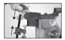
**5.** Ensure the e-clip is installed into the groove in the supplied large drill bit.
